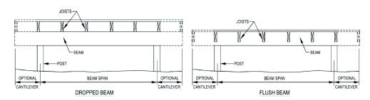
FIGURE AM105.2 TYPICAL DECK GIRDER SPANS
